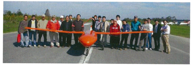
Fig.2. Josaphat Laboratory Experimental CP-SAR onboard Unmanned Aerial Vehicle (CP-SAR UAV : JX-1)
