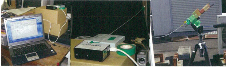
Figure 2. The direct sunlight DOAS configuration with USB2000+ Spectrometer.
