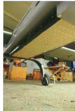
Fig.11 SAR Antenna Mounted Underneath the Fuselage
