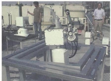
Experiment for rolling/pitching with 5-degree amplitude and 10-sec cycle simulating the actual conditions based on the characteristics of the former Antarctic R/V Shirase
