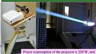
Power consumption of the projector is 220 W, and the emission covers the visible wavelength.
