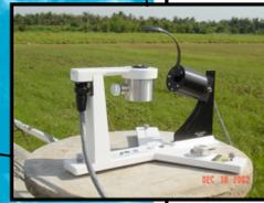
Rotating shadowband Radiometer (RSS)
