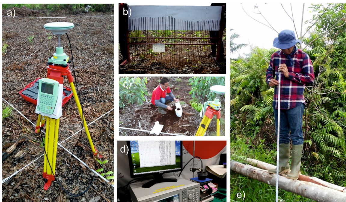
Fig 1. a) position measurement, b) soil roughness measurement, c) soil sampling, d) dielectric constant measurement, and e) groundwater table measurement
