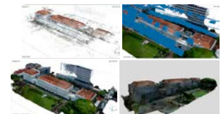
Fig.2 The process and results of the 3D scan of the Daendels Palace of Jakarta by Agisoft (August, 2024)
