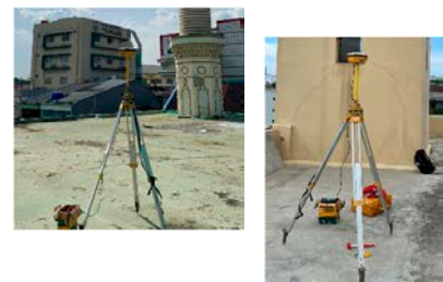
Fig.2 Ground survey measurement using GPS/GNSS
