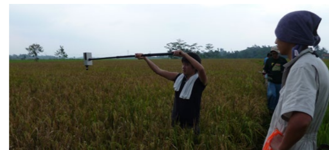
水田での分光反射計測 Measurement of spectral reflectance in paddy field
